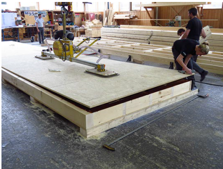
Prefabrication of the roof members in the plant of Kaufmann Bausysteme (photograph: SWISS KRONO GmbH)
