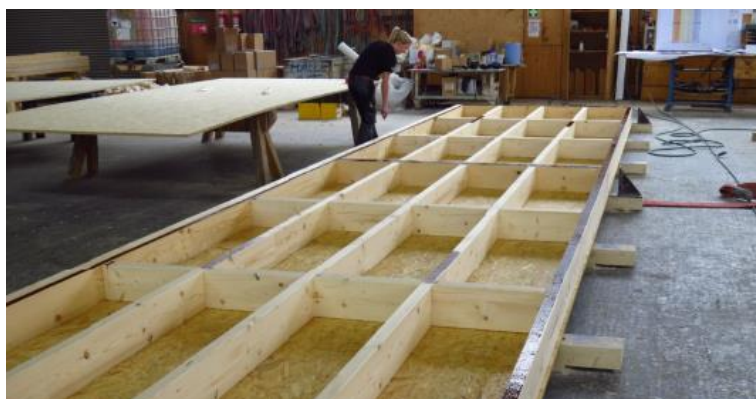
Prefabrication of the roof members in the plant of Kaufmann Bausysteme (Photo: SWISS KRONO GmbH)
